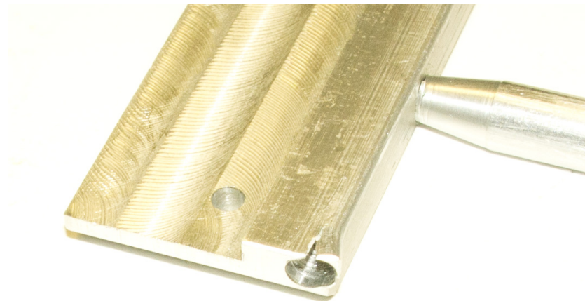
Fig. 1. Broken flat kicking plate
